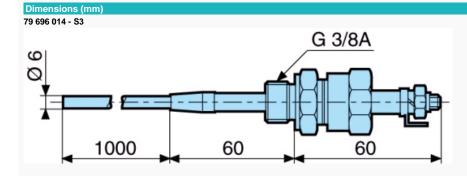
Electrode holder with a single probe supplied in a standard length of 1000mm. (304 stainless steel). Mounting with external 3/8" BSP thread and hexagonal head. Use 24 mm. spanner for hexagon. Suitable for use on boilers, autoclaves and under high temperature conditions up to 200 °C and high pressure conditions up to 25 kg/cm 2
